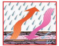
**Excessive energy costs.**Possible cause: Insufficient attic ventilation causes heating/cooling system to run excessively.
