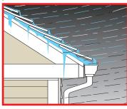
Leakage in attic after driving rain.
