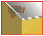
Stains on interior ceilings and walls or mold and mildew growth. Possible cause: Inadequate or faulty shingle underlayment allowing leakage, or inadequate ventilation.
